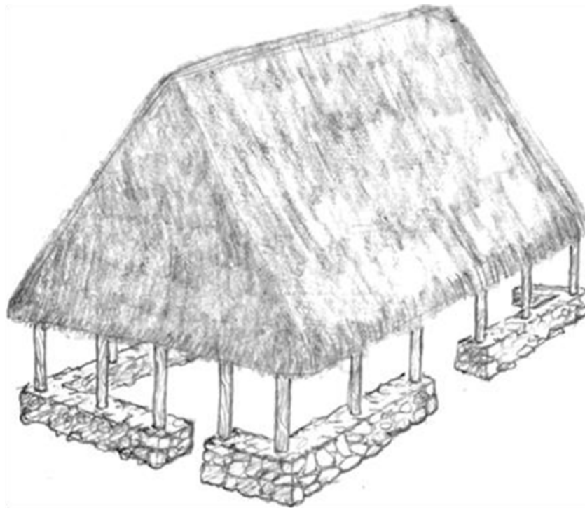
An example of a hale hālāwai. Source: APPENDIX X Hawai'i Provisions For Indigenous Hawaiian Architecture Structures section of Chapter 12 of the Kaua'i county Building code, the traditional A-frame style.
